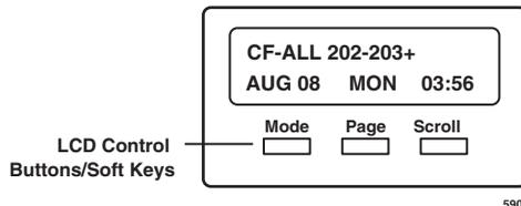
**Important!** *The LCD width of the DKT2000-series telephones is shorter than the IPTs and DKT3000-series LCDs. This difference causes some features to display differently.*
