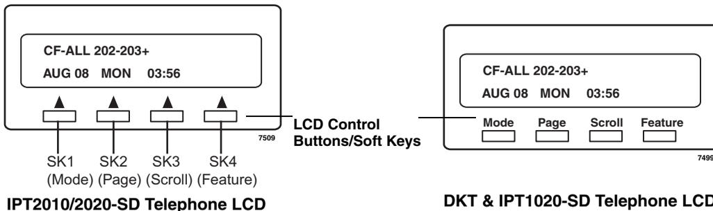
**Note** The IPT and DKT soft keys perform the same functions. This manual uses the IPT soft keys (SK) to refer to the soft keys on all telephones. For example, if an instruction references SK1, this means use the first soft key (from left to right) on the IPT and use Mode on the DKT. SK2, SK3 and SK4 equate to the second, third and fourth soft keys on the IPT or Page, Scroll and Feature on the DKT.
